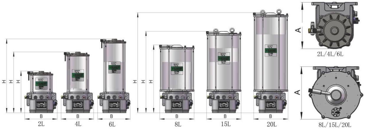
Dia. 19.1 Installation dimensions for ALPB pump reservoir, 2 to 6 Liter D170mm, 8 to 20 D230mm
